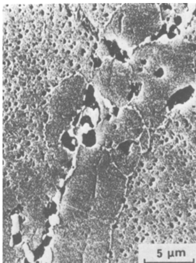
Figure 4 Recrystallized grains nucleated from coarse \gamma' . Scanning electron micrograph of the HT2 1080°C-40% forged material.
